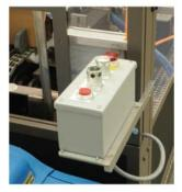
The Mach-2S case packer can be started from (two) locations (optional.) An HMI control panel is integral to the machine guarding and there is also a remote push button station.
